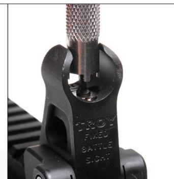
Adjustments: To move bullet impact up, turn adjustment wheel to the right/clockwise. To move bullet impact down, turn adjustment wheel to the left/counter clockwise.
