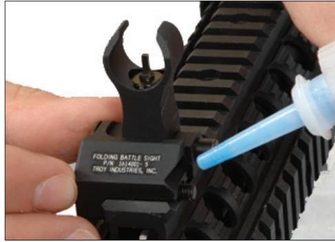
2. Apply one drop of thread locking compound to expose threads. Replace clamp and tighten screw while pushing sight forward against cross-slot.
