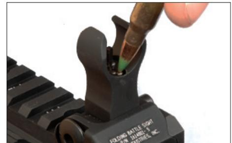
Adjustments: To move bullet impact up, turn adjustment wheel to the right/clockwise.
