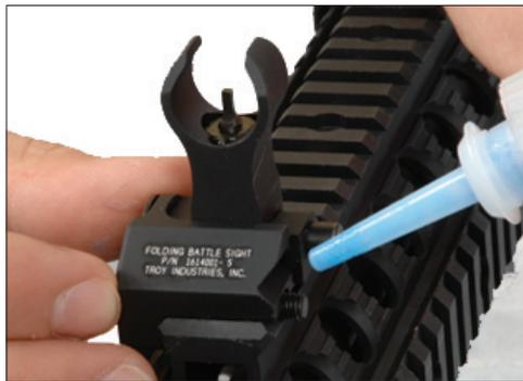
2. Apply one drop of thread locking compound to expose threads. Replace clamp and tighten screw while pushing sight forward against cross-slot.
