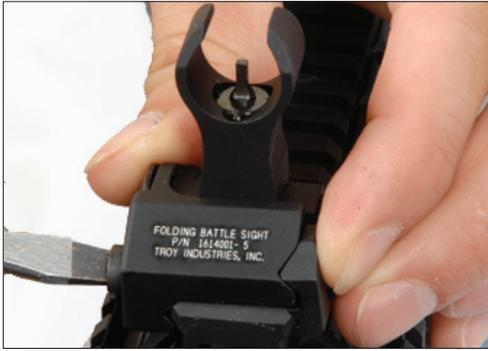
1. Unscrew clamp assembly and place sight so as to allow clamp screw to rest in foremost rail cross-slot on handguard.
