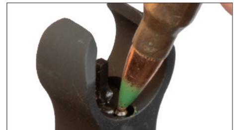
Adjustments: To move bullet impact down, turn adjustment wheel to the left/counter clockwise.
