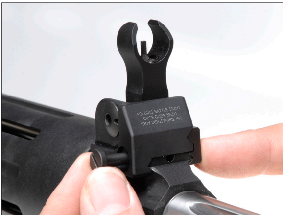
3. Replace clamp and tighten screw while pushing sight forward against cross-slot.
