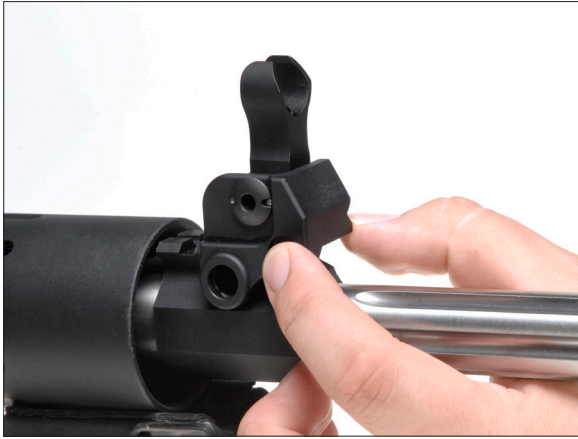
1. Unscrew clamp assembly and place sights at desired locations.
