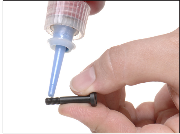
2. Apply one drop of thread locking compound to exposed threads.
