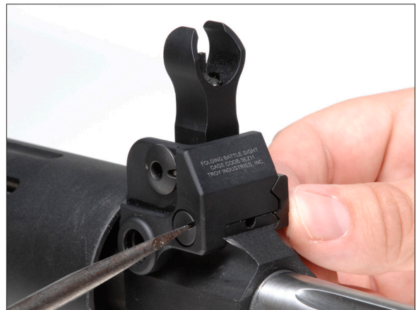
3. Replace clamp and tighten screw while pushing sight forward against cross-slot.
