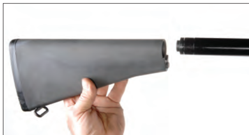
7. Slide buttstock down over receiver extension.
