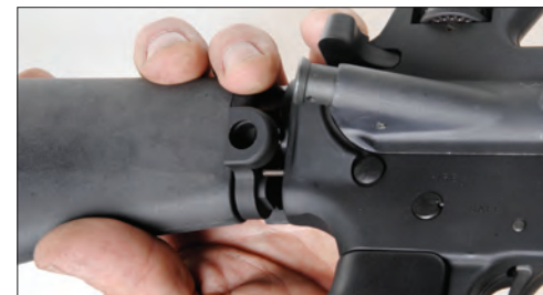
8. Slide sling mount down receiver extension. Carefully collapse rear takedown detent spring back into detent hole with sling mount and slide buttstock down against mount.
