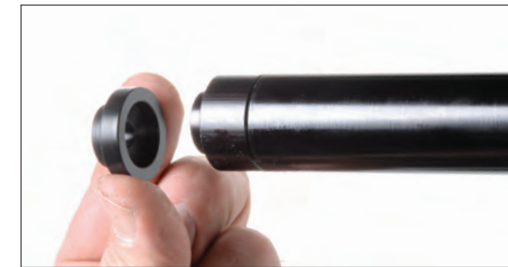
6. Install supplied stock spacer on original tube spacer. (Note: Only A2 stocks will have large spacer.)
