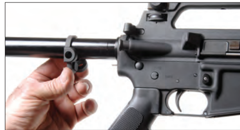
5. Slide sling mount down receiver extension with small plug facing forward.
