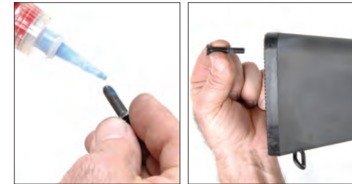
9. Put one drop of thread locking compound onto new buttstock screw. Insert screw into hole and tighten.
