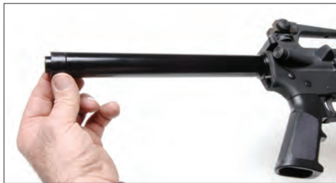
4. Make sure large stock spacer is on receiver extension. (Note: Only A2 stocks will have large spacer.)
