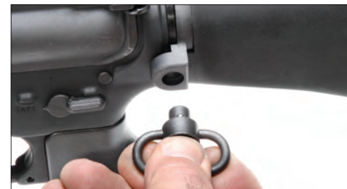
11. Depress center button of S.S.Q.D. sling adaptor and install into mount hole.
