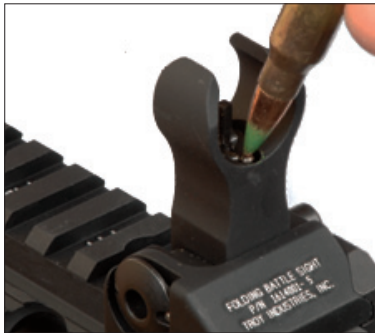
2. Apply one drop of thread locking compound to exposed threads
