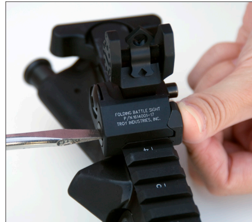
3. Replace clamp and tighten screw while pushing sight forwards against cross-slot.
