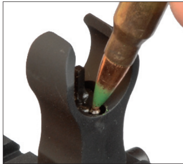
2. Apply one drop of thread locking compound to exposed threads
