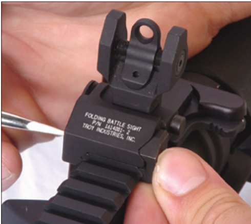
1. Unscrew clamp assembly and place sights at desired locations.
