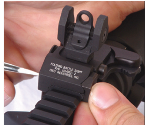
3. Replace clamp and tighten screw while pushing sight forward against cross-slot.
