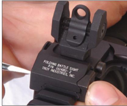
2. Apply one drop of thread locking compound to expose threads. Replace clamp and tighten screw while pushing sight forward against cross-slot.
