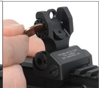
Adjustments: Can be made with a 5.56mm bullet tip (left) or a coin using the coin slot (right). To move bullet impact right, turn adjustment wheel to the right/clockwise. To move bullet impact left, turn adjustment wheel to the left/counter clockwise.
