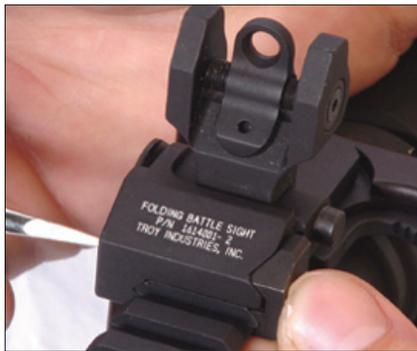
2. Apply one drop of thread locking compound to expose threads. Replace clamp and tighten screw while pushing sight forward against cross-slot.
