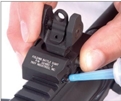
1. Unscrew clamp assembly and place sight so as to allow clamp screw to rest in foremost rail cross-slot of flat top receiver.
