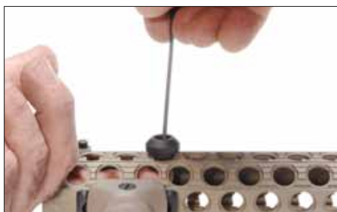
5. Place adapter into hole over retainer and tighten screw.
