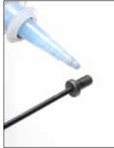
2. Put small drop of thread locking compound on screw threads. Insert screw and hex wrench into adapter.
