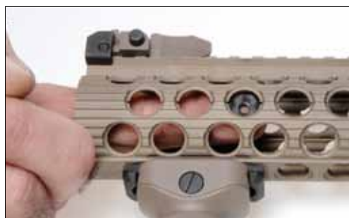
4. Place retainer under hole where you want adapter to be.
