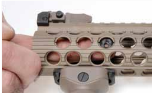
4. Place retainer under hole where you want adapter to be.
